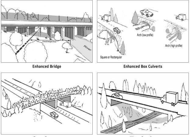
Figure 23. Schemes for Fauna Crossings—Enhanced Culverts and Bridges
