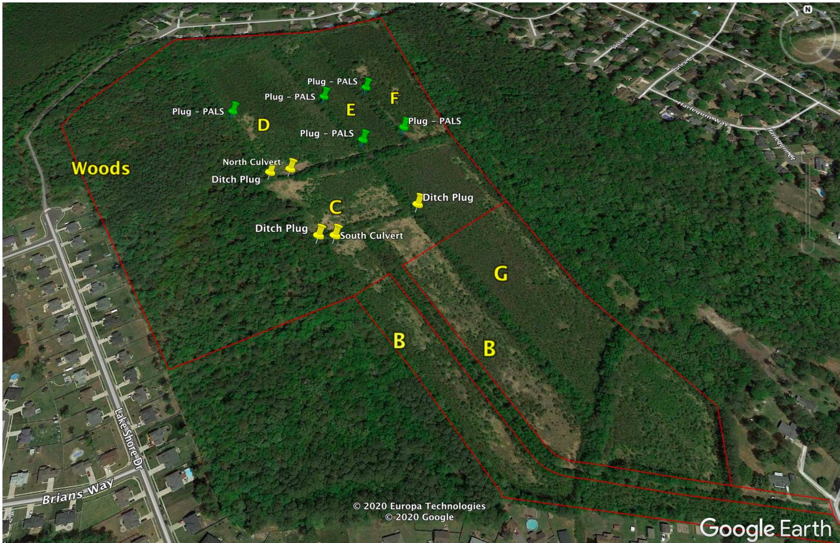
Exhibit 6. Map shows current conceptual plan for installation of PALS and permanent ditch plugs within the existing ditches.
